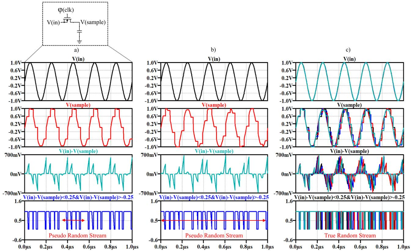
**FIGURE 2.** STAMP's entropy source generation: a) case (a), frequency of  $V(in)$  is multiple of  $\phi(clk)$ , b) case (b), frequency of  $V(in)$  is co-prime with  $\phi(clk)$ , c) case (c), frequency of  $V(in)$  is co-prime with  $\phi(clk)$  where a low-jitter occurs.
