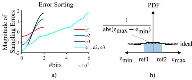
**FIGURE 4.** Sorting and PDF of sampling errors: a) sorting of sampling errors from each harmonic and sorting of mixed sampling errors (e1,e2,e3), b) PDF of mixed sampling errors.
