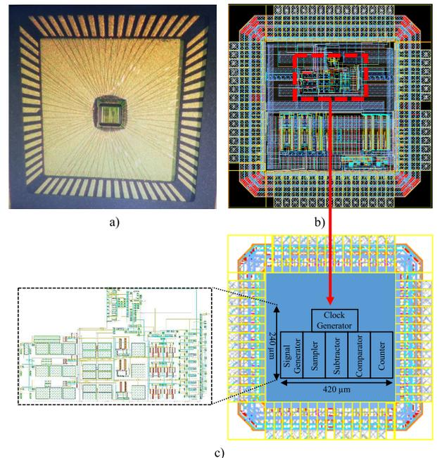
FIGURE 8. STAMP chip: a) STAMP wire bonding in CLCC 68-pin package, b) STAMP's routing, c) STAMP's block diagram and layout.
