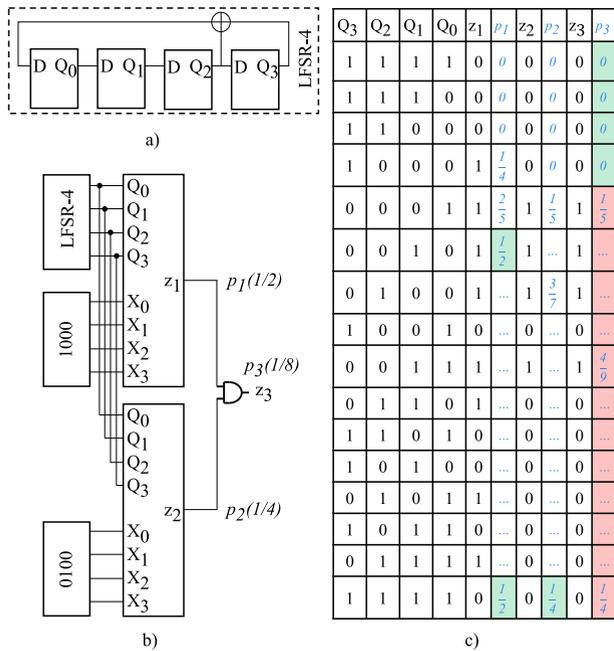
FIGURE 1. LFSR based SC circuit: a) 4-bit LFSR schematic, b) SC multiplication, c) truth table with output probabilities (p) - correct results (green), wrong results (red).
