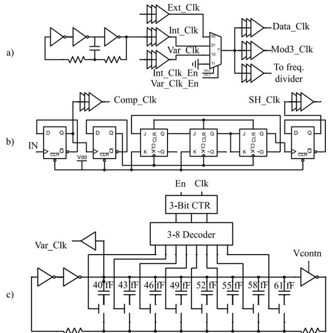
FIGURE 7. System clock generator: a) clock configuration, b) frequency division for comparator and sampling clocks, c) variable system clock generation.
