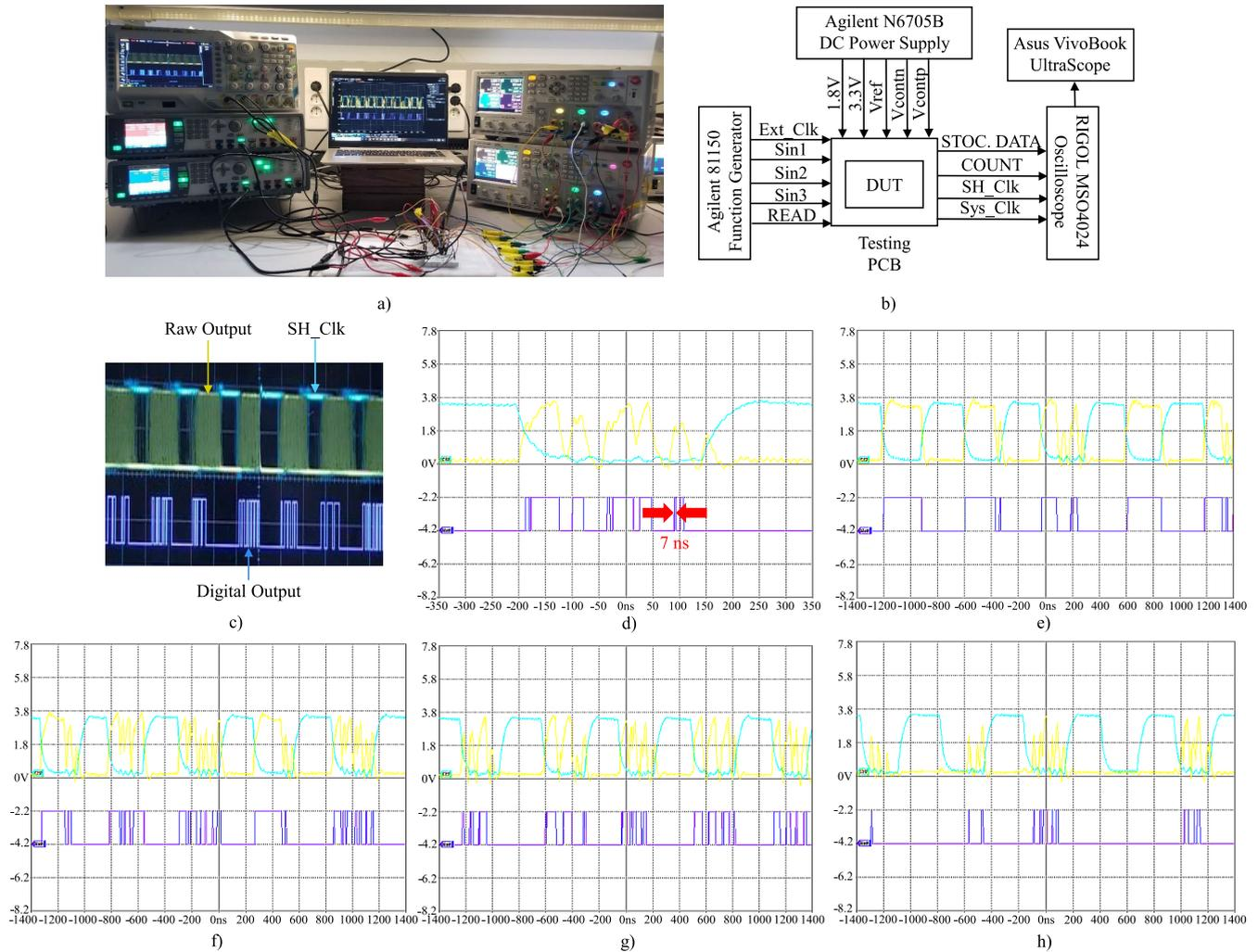
**FIGURE 9.** Test setup of STAMP: a) test setup view in VLSI Lab, b) test setup block diagram, c) oscillator output: raw output(yellow), sample and hold clock (cyan), digital output (purple), d) UltraScope views: minimum measured stochastic bit with, e-h) output waveform when Vref is set to 0.9 V, 0.75 V, 0.55 V, 0.3 V, respectively.
