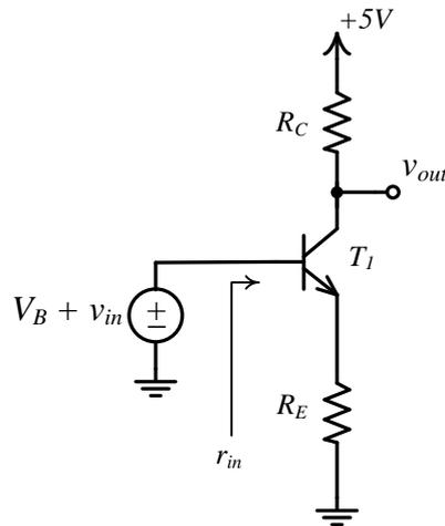
*Common Emitter Amplifier with an Emitter Resistance*
