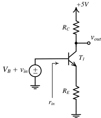
*Common Emitter Amplifier with an Emitter Resistance*
