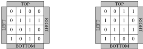
A path exists between top and bottom, f=1 No path exists between left and right, g=0
